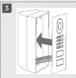
Put the front panel attached to the Main Eletrical Unit on the mounting housing.
