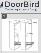
Screw the mounting housing to the adapter.
